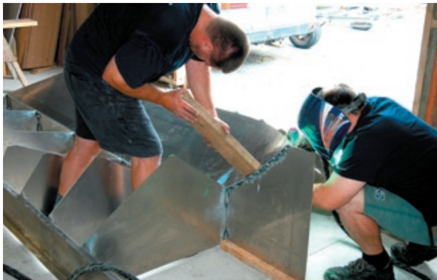
Crucial fit. Panels are tack-welded on aluminium jig, but strapped to customwood jig.
