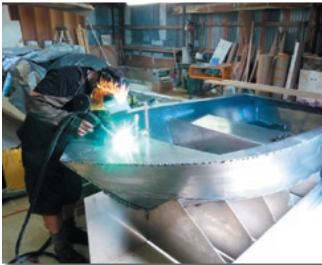
Deck tack welded.
