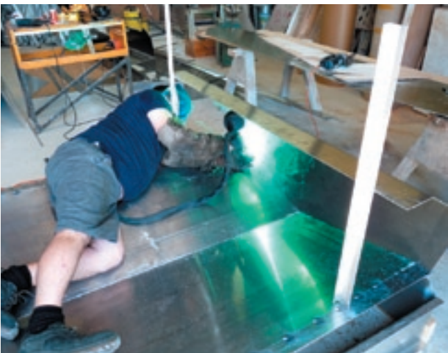
Tack welding the transom.
