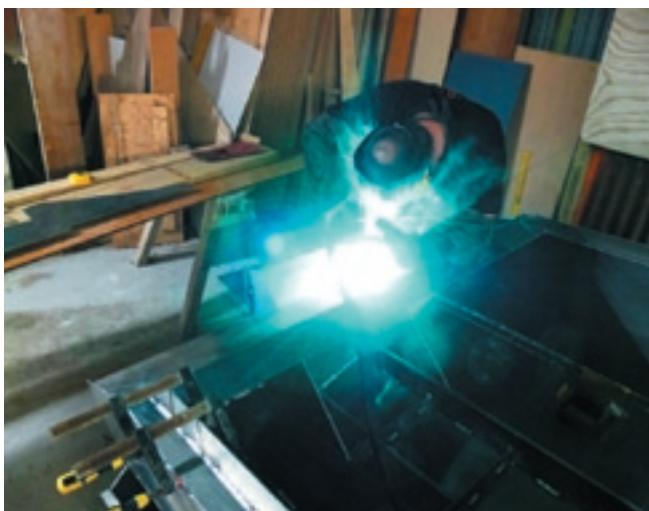
Welding outboard bracket.
