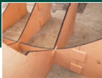
Interlocking customwood jig detail.
