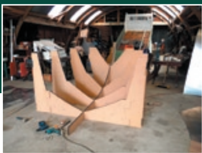
Customwood jig being set up.
